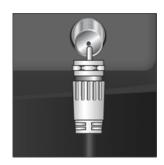
• Connect the CATV cable or TV antenna cable to the "ANT IN" port on the rear side of the product. Make sure to use a TV antenna cable (sold separately) as the antenna cable.
